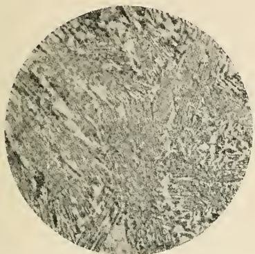
Fig. 7—Eutectic alloys of antimony and copper
